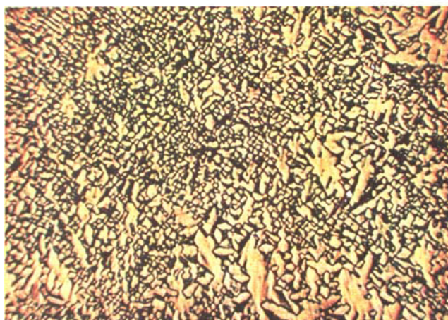
Figure 4. Field-induced focal conic texture. Crossed polarisers, white light, magnification 200\times .
